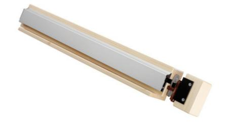
A range of drop down seals for the bottom of doors also know as dropseals. The seals are activated by the closing action of the door dropping down to seal only when the door is closed. This leaves the threshold clear and flat without the need for high fixed thresholds. These seals have been tested without threshold plates and also straight down to carpet.
