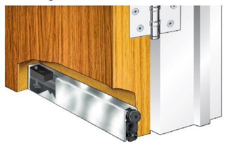
A range of drop down seals for the bottom of doors also know as dropseals. The seals are activated by the closing action of the door dropping down to seal only when the door is closed. This leaves the threshold clear and flat without the need for high fixed thresholds. These seals have been tested without threshold plates and also straight down to carpet.
