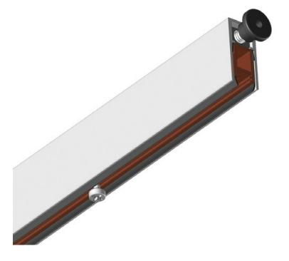
A range of drop down seals for the bottom of doors also know as dropseals. The seals are activated by the closing action of the door dropping down to seal only when the door is closed. This leaves the threshold clear and flat without the need for high fixed thresholds. These seals have been tested without threshold plates and also straight down to carpet.
