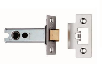
Heavy Sprung Tubular Latch. 76mm with an 8mm Follower. Ideal for unsprung knobs or handles. The cut away holes in the body allow for bolt through fittings ensuring a secure fixing.
