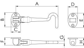
Versatile hook and eye pattern. Most commonly used on doors and window shutters. Available in 2 finishes and 3 sizes. It provides the perfect solution to restricting doors or gate movement, and can prove to be a more visually appealing option to that of the average bolt.
