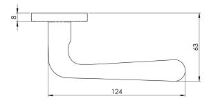
Lever on concealed fix press on round rose. The smooth round lever has a slender middle expanding slightly to the end. Part of the Steelworx Grade 304 stainless steel range. Comes with a 10 year mechanical guarantee and is Fire door rated.
