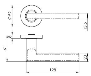
Lever on concealed fix press on round rose. A straight smooth round bar lever on rose. Part of the Steelworx Grade 304 stainless steel range. Comes with a 10 year mechanical guarantee and is Fire door rated.
