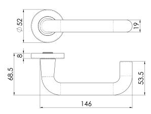
A sturdy 19m Dia. round bar safety lever on a concealed fix press on round sprung rose. The handle returns back to the door offering reduced risk of catching clothes or injury. DDA Compliant.
