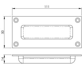
Rectangular flush pull mainly used on sliding doors. A modern style recessed box flush pull. The main cup is recessed into the door to leave a flush appearance. Suitable for domestic and commercial use.
