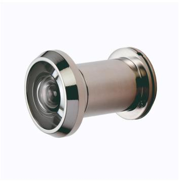
Door Viewer 200 degree with Crystal lens. Standard style door viewer adds a useful security aspect to any door by enabling the user to see who is on the other side of the door before opening it. Extends to suit doors 35 - 60mm deep. For wider doors up to 100mm an extension sleeve (SWE1011) is available.
