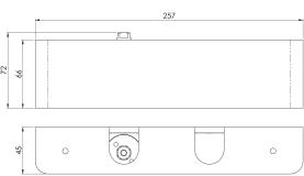
Electromagnetic HO/FS Door Closer Variable Power Size 2-4. Carries the CE mark and is certified to BS EN 1154, BS EN 1155 and BS 8300 to meet the needs of disabled people. Comes with a 2 year electrical guarantee, a 10 year mechanical guarantee and is Fire door rated. Suitable for all domestic, commercial and industrial use.
