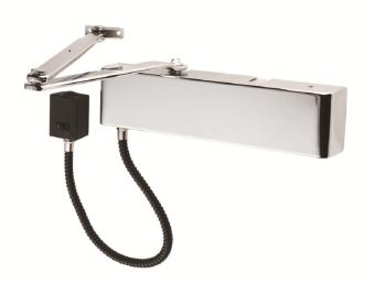
Electromagnetic HO/FS Door Closer Fixed Power Size 3. Carries the CE mark and is certified to BS EN 1154, BS EN 1155 and BS 8300 to meet the needs of disabled people. Comes with a 2 year electrical guarantee, a 10 year mechanical guarantee and is Fire door rated. Suitable for all domestic, commercial and industrial use.
