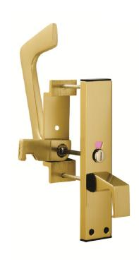
DDA Compliant Disabled Toilet Handle Set (Dual Handed). A versatile handle assembly, suitable for hinged/swing or sliding doors offering easy access with a simple lever operation. It also has a reversible function allowing the user to choose for a left or right hand opening, complete with a coin release on the outside which can be operated in case of emergencies and a coloured indicator denoting vacant or engaged. Comes with a 10 year mechanical guarantee.
