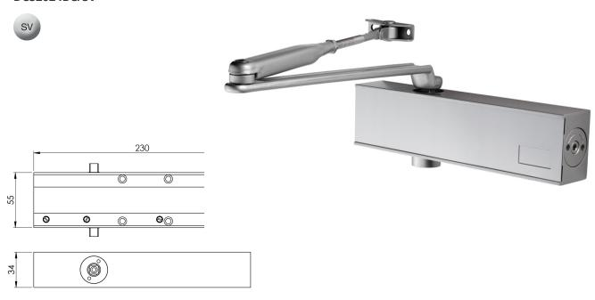
Overhead Door Closer Variable Power Size 2-4. Certified to BS EN 1125 and BS 8300 to meet the needs of disabled people. CE marked and Certifire tested. Comes with a 10 year mechanical guarantee and is Fire door rated.
