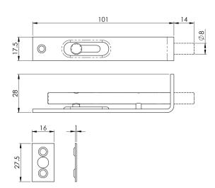
A perfect solution for providing additional home security. In contrast to the standard flick lever action flush bolt this function is operated by sliding the shoot using the small knob. Supplied with flat keep plate and fixings. Comes with a 10 year mechanical guarantee.
