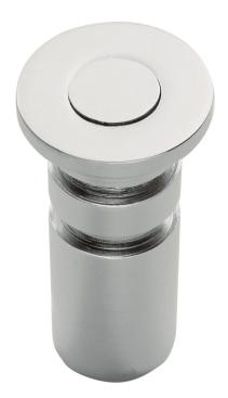
For insertion in concrete floors, spring loaded dust cover. These sockets are designed to accept the shoot of a flush bolt, and have a sprung central section which will depress when the flush bolt is engaged. When the flush bolt is disengaged, the sprung section will return flush to the top of the plate, thus stopping dust and dirt falling into the hole. Ideal for concrete floors in areas where a traditional flush bolt plate would gradually fill up and trap debris from the floor.
