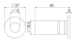
For insertion in concrete floors, spring loaded dust cover. These sockets are designed to accept the shoot of a flush bolt, and have a sprung central section which will depress when the flush bolt is engaged. When the flush bolt is disengaged, the sprung section will return flush to the top of the plate, thus stopping dust and dirt falling into the hole. Ideal for concrete floors in areas where a traditional flush bolt plate would gradually fill up and trap debris from the floor.
