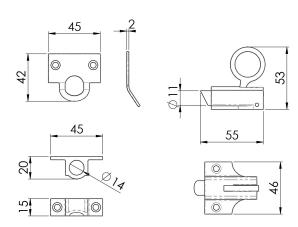
A sprung fanlight catch, mainly for use on bottom hung casement windows. The sprung loop allows high level windows to be reached with a hook-on-a-pole. Can also be used on doors, cabinets etc. Supplied with fixings, flat plate and receiver staple.
