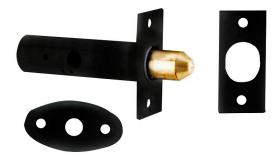
Contract Door Security Bolt, sometimes called a Rack Bolt. The bolt is morticed inside the door edge and can be locked or unlocked via a separate splined key or with a fixed splined turn. The bolt has an internal sawtooth rack mechanism into which the splined key is inserted. The spline engages with the rack teeth and forms a gearing action which smoothly operates the bolt.
