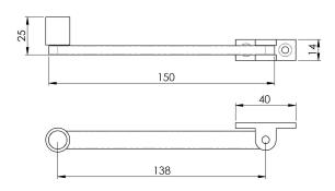
The roller arm stay is used to restrict the opening of light to medium weight bottom hung fan light windows and side hung windows. Fitted with a brass roller ensuring longevity in service unlike the cheaper plastic rollers. The roller is plated to match the arm finish. The stay can be used individually or in pairs depending on width of window.
