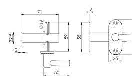
Security bolt with a cylindrical turn lever on a radius backplate. By rotating the small turn handle it engages the teeth on the bolt and slides it out smoothly from its housing into the opposing plate on the door frame, thereby locking the door. Reversing direction of handle retracts it back into position. Provides additional security, convenient and easy to use.
