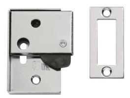
To aid locking of self-closing doors in a simple operation. As the door closes the cam is lifted up by the tubular latch and then falls behind it securing the door in the closed position. To release and open the door, simply depress the door lever handle to retract the latch.
