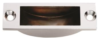
The socket can be placed in the floor to allow the door to be secured in a closed or open position when used in conjunction with flush or surface door bolts. The internal curvature enables easy cleaning and allows the door bolt to easily engage into the socket.
