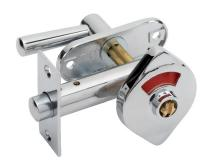
An all in one bathroom / toilet lock assembly which offers a large robust bolt which will wind into the door frame with a turn of the thumb lever. The outer case has a red/green indicator as a visual signal to show if the room is vacant or engaged. Ideal for commercial offices where toilets are shared. Emergency coin slot allows release operation of lock in an emergency.
