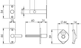
An all in one bathroom / toilet lock assembly which offers a large robust bolt which will wind into the door frame with a turn of the thumb lever. The outer case has a red/green indicator as a visual signal to show if the room is vacant or engaged. Ideal for commercial offices where toilets are shared. Emergency coin slot allows release operation of lock in an emergency.
