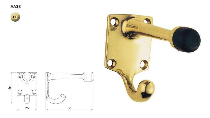
One piece hat and coat hook with rubber buffered end to protect the door. The hat hook with the buffer tip extends straight out and the coat hook is suspended below the base plate which has 4 anchor points for a secure fixing.carlislebrass.
