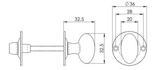
Oval shaped thumb turn with coin release for use with a bathroom lock. Comes with a 10 year mechanical guarantee.
