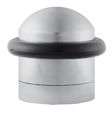
Dome top with a substantial rubber circumference to protect doors. Concealed fixing. The lower section is screwed into the floor and the top is threaded into the base. Comes with a 10 year mechanical guarantee.
