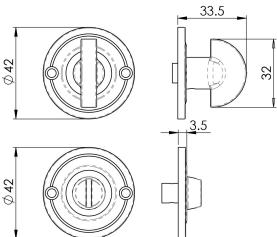
Bathroom turn and release set to compliment the Delamain door knob range. Its 42mm diameter means you can use these with the Delamain Knobs knowing that if used with a standard bathroom lock, they will fit. (the larger DK12 will not fit - use of a separate deadbolt is required) .Comes with a 10 year mechanical guarantee.
