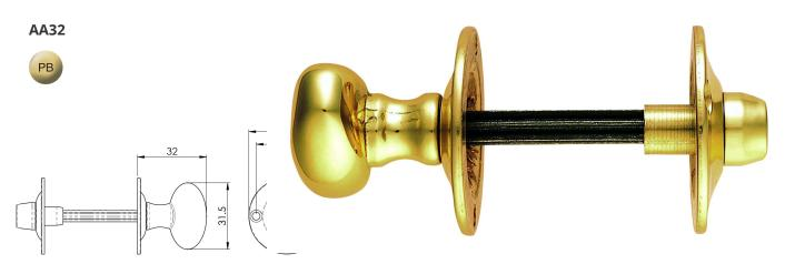
Oval thumb turn with coin release on opposing side. Splined spindle for operation with rack bolts. Progressive turning of the oval turn will move the dead bolt. Comes with a 10 year mechanical guarantee.
