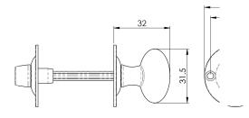
Oval thumb turn with coin release on opposing side. Splined spindle for operation with rack bolts. Progressive turning of the oval turn will move the dead bolt. Comes with a 10 year mechanical guarantee.
