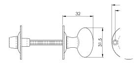
Oval thumb turn with coin release on opposing side. Splined spindle for operation with rack bolts. Progressive turning of the oval turn will move the dead bolt. Comes with a 10 year mechanical guarantee.
