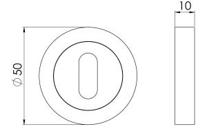
A modernistic concealed fix standard keyhole profile escutcheon with a threaded screw on outer rose. The inner rose has numerous fixing points accommodating bolt through fixings as well as conventional screws. This 50mm x 10mm thick escutcheon provides an excellent accompaniment to substantial levers on rose.
