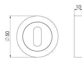
A modernistic concealed fix standard keyhole profile escutcheon with a threaded screw on outer rose. The inner rose has numerous fixing points accommodating bolt through fixings as well as conventional screws. This 50mm x 10mm thick escutcheon provides an excellent accompaniment to substantial levers on rose.
