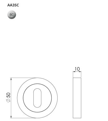
A modernistic concealed fix standard keyhole profile escutcheon with a threaded screw on outer rose. The inner rose has numerous fixing points accommodating bolt through fixings as well as conventional screws. This 50mm x 10mm thick escutcheon provides an excellent accompaniment to substantial levers on rose.
