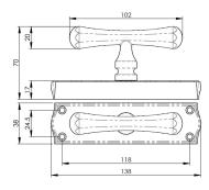
T-Bar style handle espagnolette bolt used for securing a door top and bottom by simply turning the handle. They are used on French doors and have a strong visual presence being surface mounted and provide additional security. To suit inward and outward opening doors, comes with 2 x 1.2m Rods and Mortice Keepers to suit a variety of applications.
