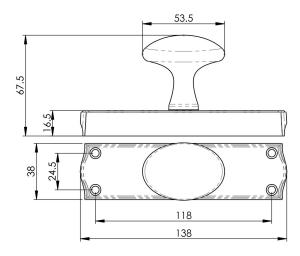
Oval knob style handle espagnolette bolt used for securing a door top and bottom by simply turning the handle. They are used on French doors and have a strong visual presence being surface mounted and provide additional security. To suit inward and outward opening doors, comes with 2 x 1.2m Rods and Mortice Keepers to suit a variety of applications.
