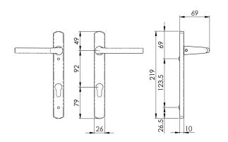
A simple straight lever on a Euro lock narrow backplate. It has a Euro profile keyhole 92mm c/c and operates a multipoint lock. Comes with a 10 year mechanical guarantee. Suitable for domestic and commercial use.
