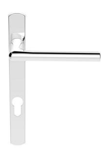
A simple straight lever on a Euro lock narrow backplate. It has a Euro profile keyhole 92mm c/c and operates a multipoint lock. Comes with a 10 year mechanical guarantee. Suitable for domestic and commercial use.
