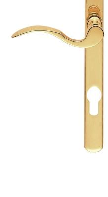
Fashionable, traditional style scroll lever on a Euro lock narrow backplate. It has a Euro profile keyhole and operates a multipoint lock. This handle is handed depending on which side the door is hinged and whether inward or outward opening. The right or left option will need to be specified when ordering.
