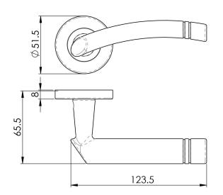
Lever on a concealed fix press on round rose. The Cuarenta lever on rose features etched rings detailed at the end with a gentle curved handle which fits nicely into the palm of the hand. Comes with a 10 year mechanical guarantee and is Fire door rated. Suitable for domestic and commercial use.
