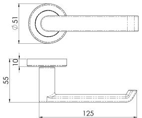
Lever on a concealed fix 2 part screw on round rose. A favoured design for the commercial environment is the Concept lever. The bold face of the lever and return to door feature gives visual impact along with safety. The chamfered edge concealed fix rose reflects the attention to detail in this range.
