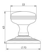
A simple classic smooth ringed knob. Featuring a ringed pattern around the knob & rose. The knob is mounted on a concealed fix rose thus no fixings are visible. Comes with a 10 year mechanical guarantee.
