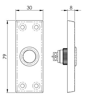
The classical door bell push will compliment most front doors. Its unobtrusive low profile button push sits on a rectangular plate which has four fixing points providing a secure and solid fitting. Comes with a 10 year mechanical guarantee.
