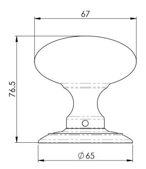
Large rounded mortice knob. Visually appealing this smooth mortice knob is comfortable to grip and operate. Its simplicity makes it very versatile for use in both contemporary and traditional settings. The knob is mounted on a concealed fix tiered rose thus no fixings are visible.
