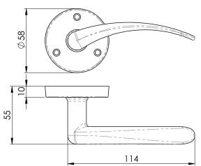
An elegant slim curved lever on a round rose. The arched lever handle features a sleek curve, thinning out towards the end for a comfortable and ergonomic grip. The three point fixing provides secure and easy installation. A contemporary door handle that features a sophisticated and chic design.
