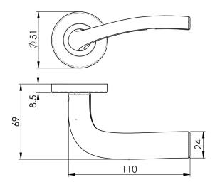
Lever on a concealed fix press on round rose. The slightly raised lever is almost flat with curved and smooth edges. Simple and ergonomic handle ideal for residential or commercial use. Comes with a 10 year mechanical guarantee and is Fire door rated.
