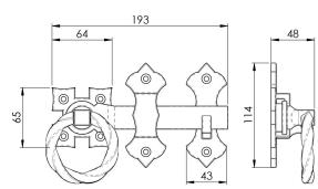
Black Antique basic ring handle gate latch. When the ring handle is lifted and turned this raises the latch bar from its keep allowing the gate to open. Comes with a 10 year mechanical guarantee. Ludlow Black Antique is a traditional range of furniture with a powder coated Black finish.
