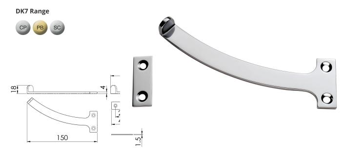
The Quadrant arm window stay is generally used to restrict the opening of bottom hung fan light or casement windows. When fitted the quadrant stays will only allow the window to open a fixed safe distance. Usually they are fitted in pairs, mainly used for bottom hung casement windows, supporting the casement as it falls inwards. Comes with a 10 year mechanical guarantee.
