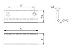
Wide style sash lift. A necessary fitting to lift the bottom sliding sash window up manually. Two lifts should be fitted, one on either side of the window. The ergonomic curves allow ample room for fingers to effect a good purchase.
