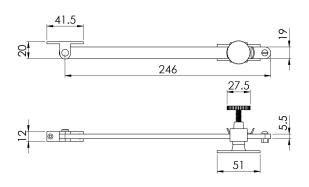
Screw down pattern casement stay is normally used to restrict the opening of windows. It can be secured in any position by screwing down the knob which clamps the arm. Comes with a 10 year mechanical guarantee.
