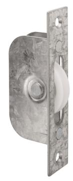
Sash window axle pulley with galvanised square forend and a nylon wheel. A range of sturdy axle pulleys for sliding sash windows. Sash window axle pulleys are used in traditional rise and fall sash windows to carry the cord attached to the window counter balance sash weight. Typically you will find four in any sash window, two for the top sash and two for the bottom sash.
