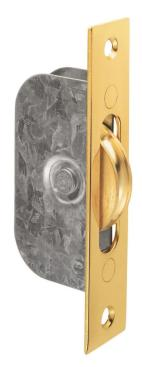
Sash window axle pulley with square brass forend and a brass wheel. A range of sturdy axle pulleys for sliding sash windows. Sash window axle pulleys are used in traditional rise and fall sash windows to carry the cord attached to the window counter balance sash weight. Typically you will find four in any sash window, two for the top sash and two for the bottom sash.
